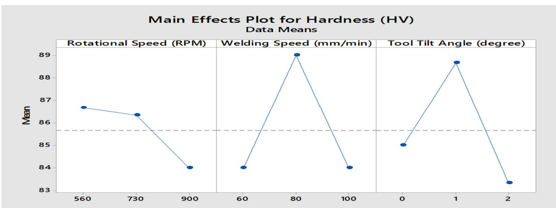
Fig 5.3 Main effects plot for Hardness (HV)
