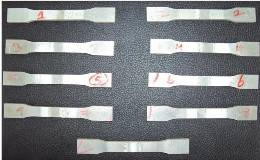
Fig 4.3 Tensile test specimens taken out of the welded plates
