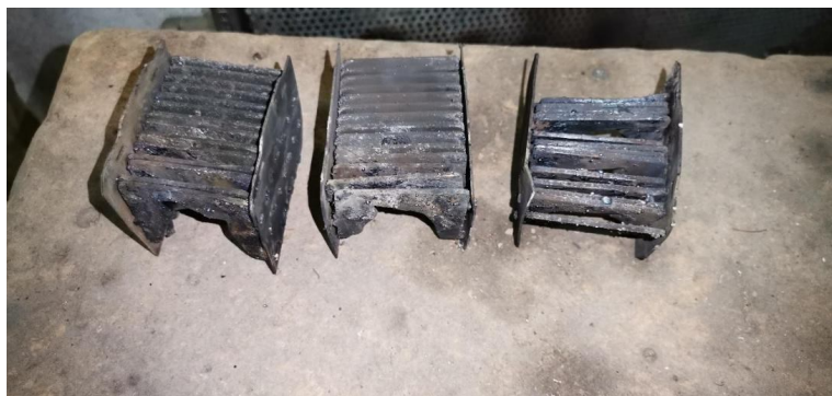
Fig. 9. Sample Separator Damage
