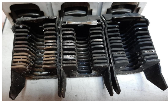
Fig. 7. Damage in Separators of Limiter-Equipped Circuit Breakers
