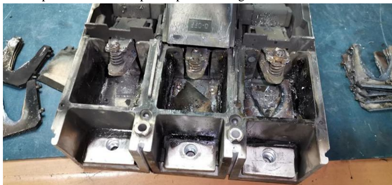
Fig. 10. Effect of Separator Changes on Arc in the Sample
