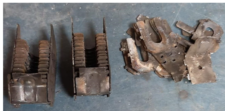
Fig. 5. Damage in Separators of Non-Limiter Circuit Breakers
