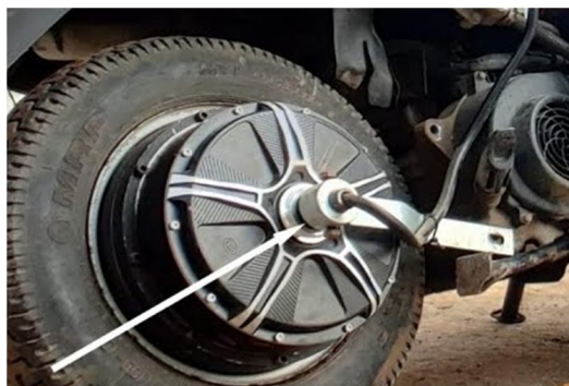
Fig.1 Two wheeler coupled with hub motor
