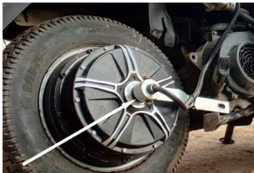
Fig.1 Two wheeler coupled with hub motor
