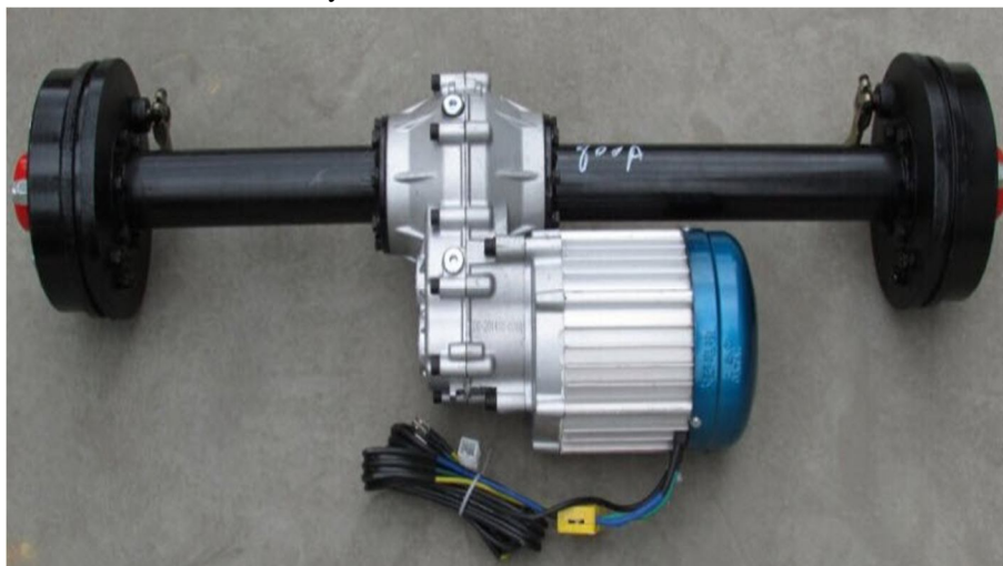
Fig.3 BLDC Motor coupled to Differential and fitted to car rear wheels
