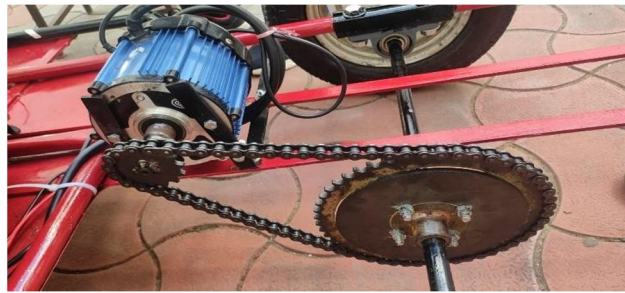
Fig 4. Mechanical connection of BLDC motor
