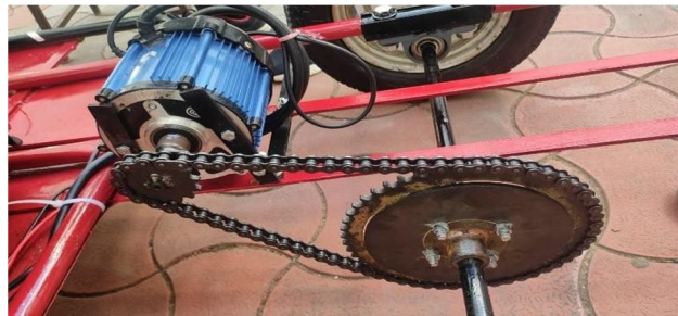
Fig 4. Mechanical connection of BLDC motor
