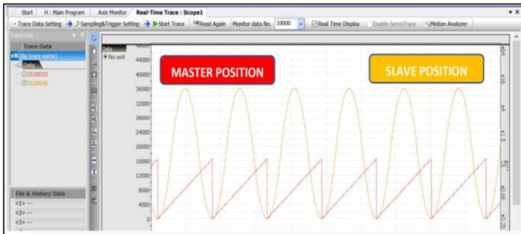
Fig. 8 Real-Time Trace of Master & slave position data
