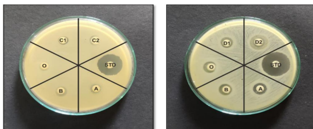
Figure 6. Zone of inhibition against S. aureus , of camphor, CNC, CNC stabilized AO-PE, and camphor-loaded AO-PEs for 40 mg and 100 mg of camphor in 15 ml of PEs, respectively.
