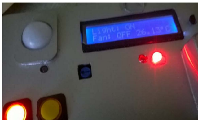
Figure 5: Device during Test(only lamp is 'on')
