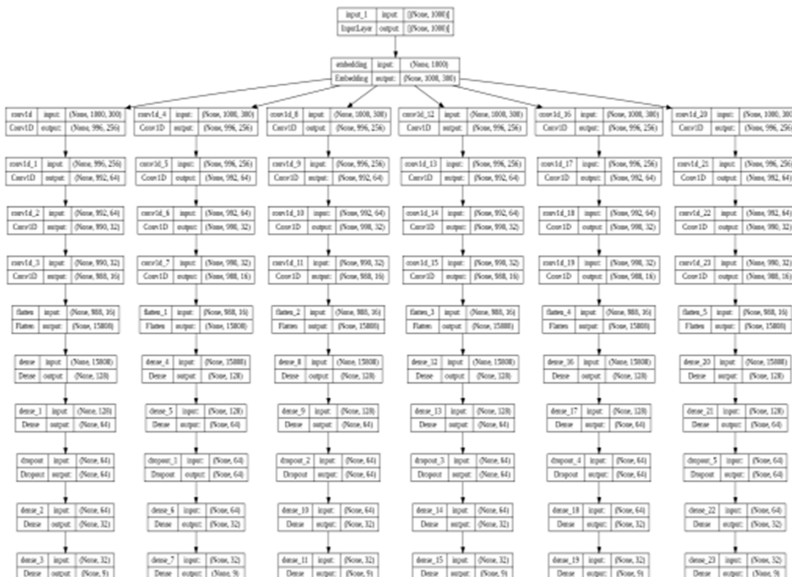
Figure 13 : embedding layer connected to 6 different Convolutional layer
