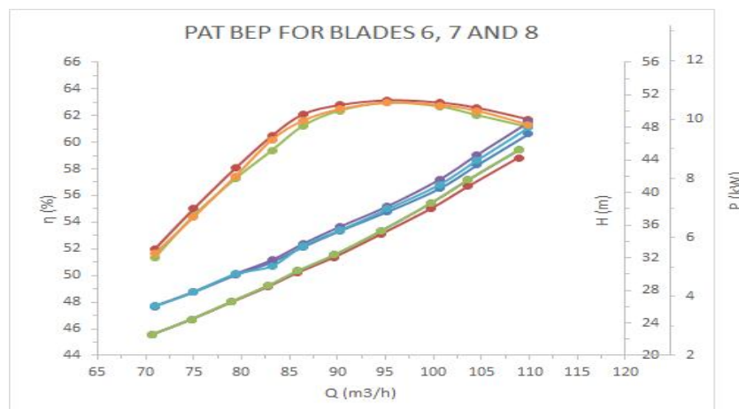
Fig. 4 comparative BEP result for PAT for Ø255
