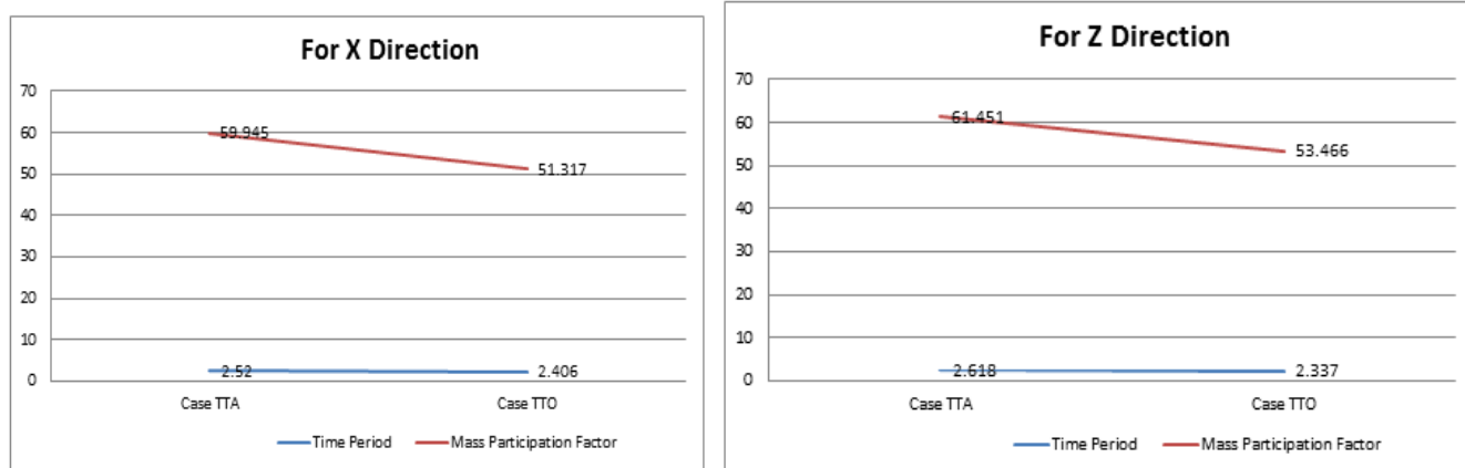
Fig. 22: Time Period and Mass Participation Factor in X and Z direction obtained in Worst Case and Erected Case
