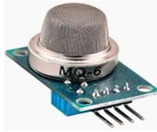
Fig 2: -MQ6 Gas sensor [8]
