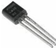
Fig 4: - Temperature sensor (LM-35)
