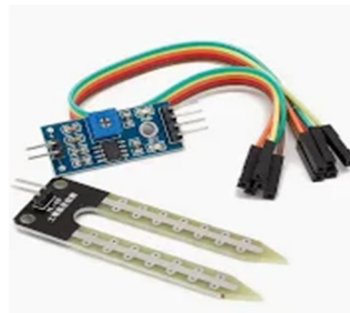
Fig 3: - soil moisture sensor (SMS) [9]
