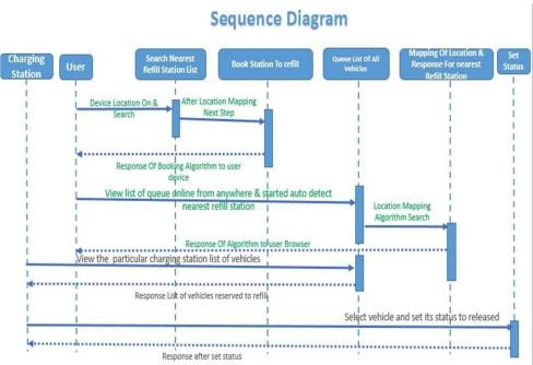
The sequence diagram explains step-by-step interactions. For example, when a user books a charging slot, the app sends the request to the backend, which checks availability with the station system and updates the database. Once the slot is confirmed, a notification is sent to the user, ensuring they have a reserved spot
