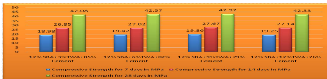
Graph 2 Relation between optimum SBA (12%) +%TWA replacement and Compressive strength
