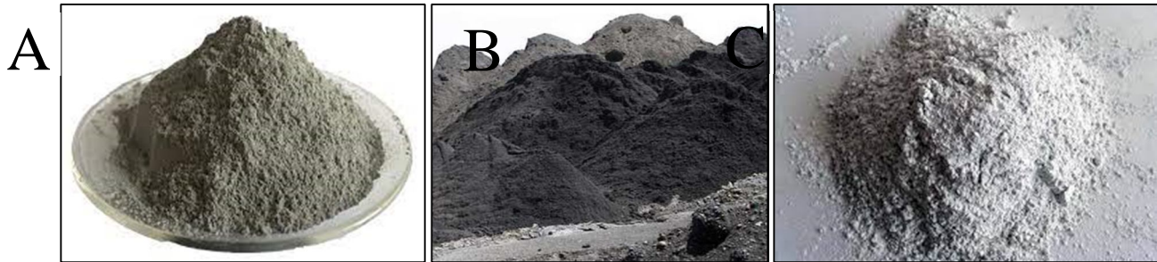
Fig. 1 Material for Soil Stabilisation (a) Silica Fume (b) Fly Ash (c) GGBS
