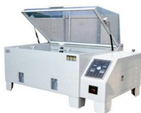
Figure:5 Corrosion (Salt Spray Testing Tub)
