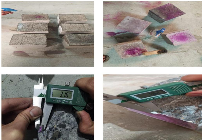
Fig. 7 Carbonation Depth Test: (As per IS-516(Part 5/Sec 3):2021
