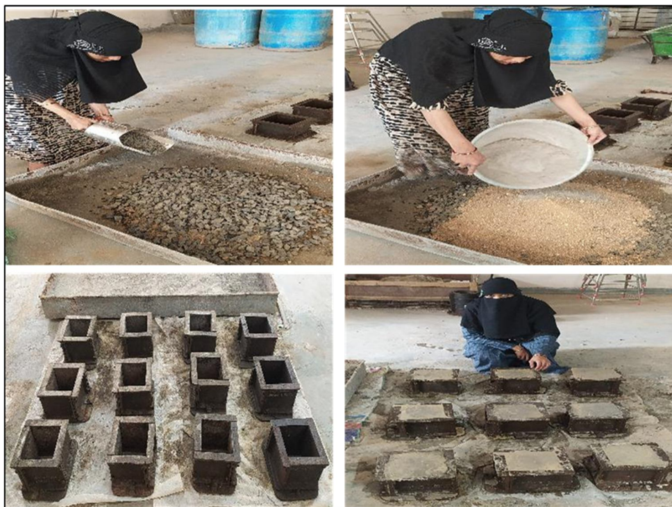
Fig. 1 Mix preparation and specimen casting
