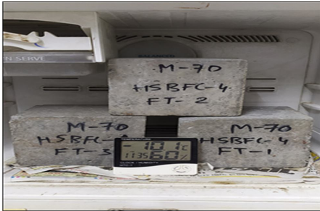
Fig. 13 Freeze–Thaw Tests of Concrete: (ASTM-C 666/C 666M – 03)
