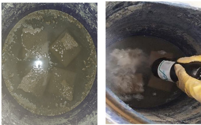
Fig. 11 Hydrochloric acid attack: As per ASTM C1898 – 20: Fig. 12 Average Comp. strength loss (%) Result after Acid attack
