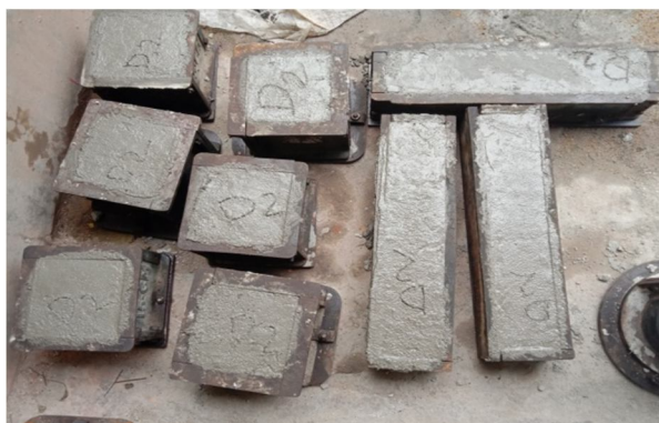
Fig 1 Casting of specimens
