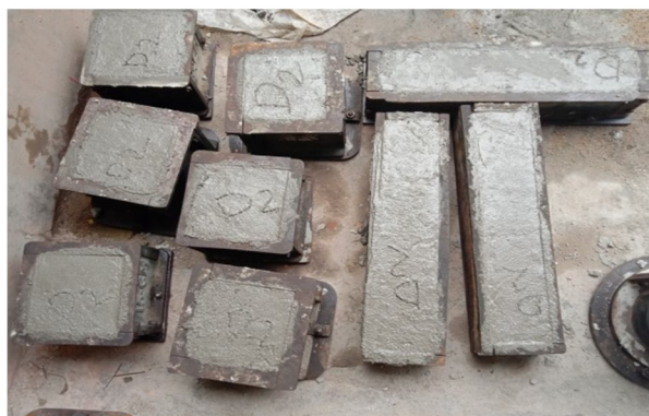
Fig 1 Casting of specimens
