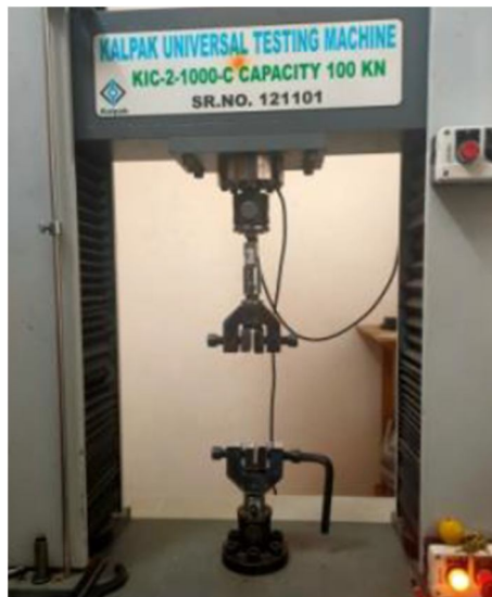
Fig 2. (a) Universal testing machine: (b) Izod testing equipment
