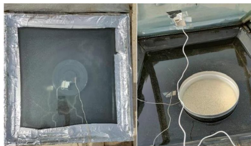
Figure 6 Solar cooker using water as TES
