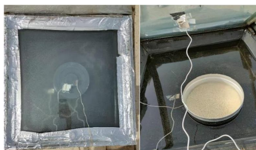
Figure 6 Solar cooker using water as TES
