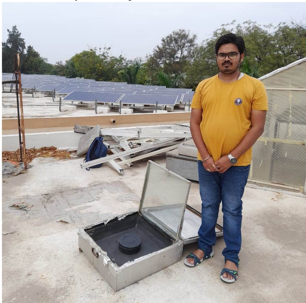
Figure 1 Solar cooker setup without TES
