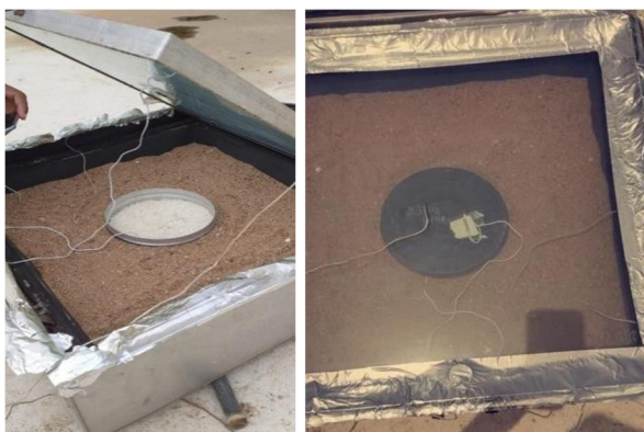
Figure 5 Solar cooker with sand as TES
