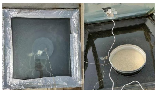
Figure 6 Solar cooker using water as TES
