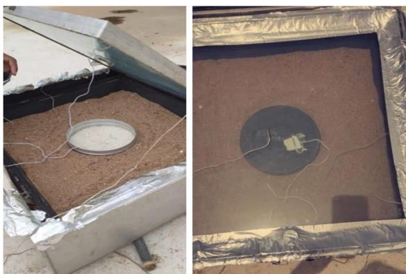
Figure 5 Solar cooker with sand as TES
