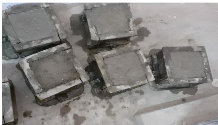
Fig 20: Cubes after Filled with concrete
