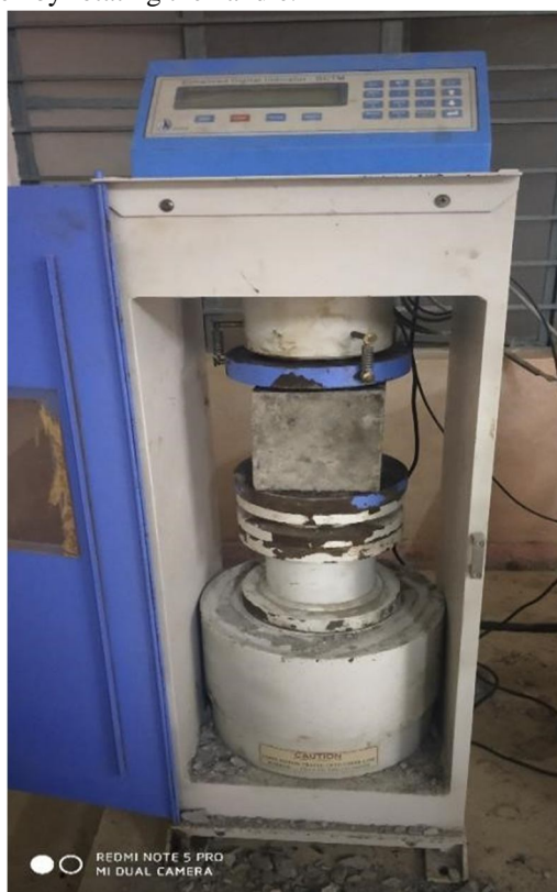
Fig 27: placing specimen for compression value
