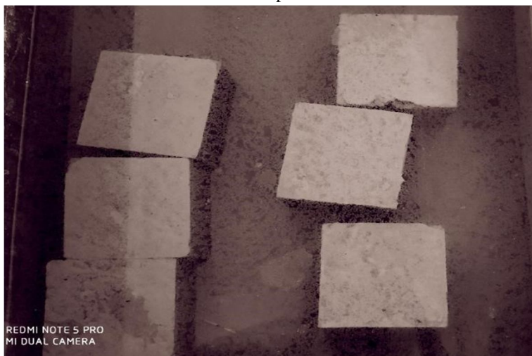
Fig 21: Cubes in Curing Tank
