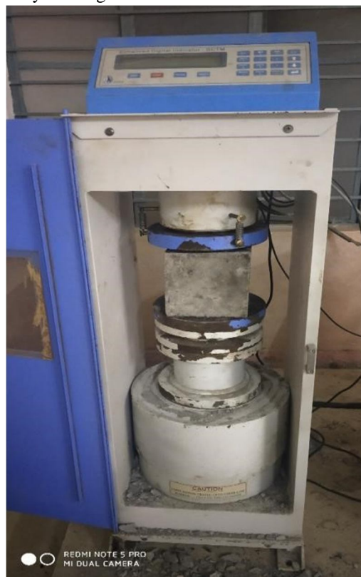
Fig 27: placing specimen for compression value
