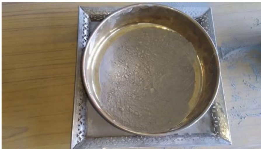
Fig 7: Fineness of Cement using 90µmm sieve
