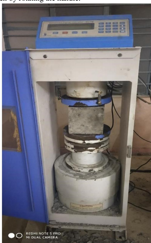
Fig 27: placing specimen for compression value
