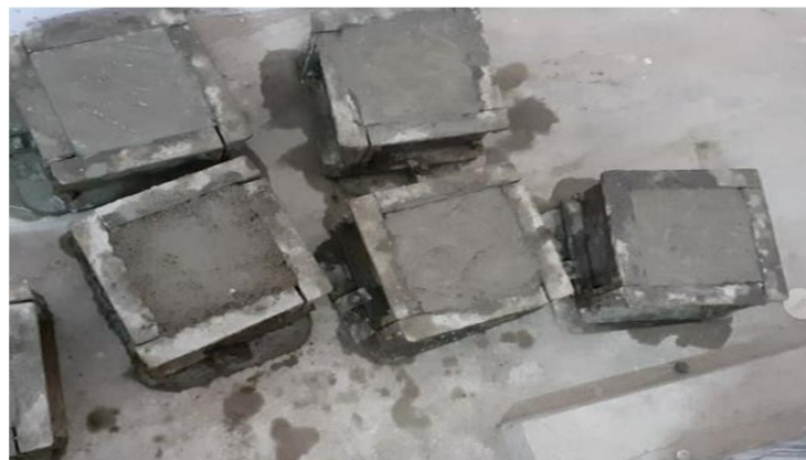
Fig 20: Cubes after Filled with concrete
