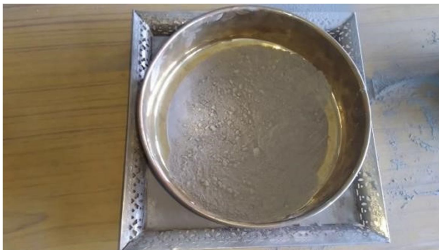
Fig 7: Fineness of Cement using 90µmm sieve
