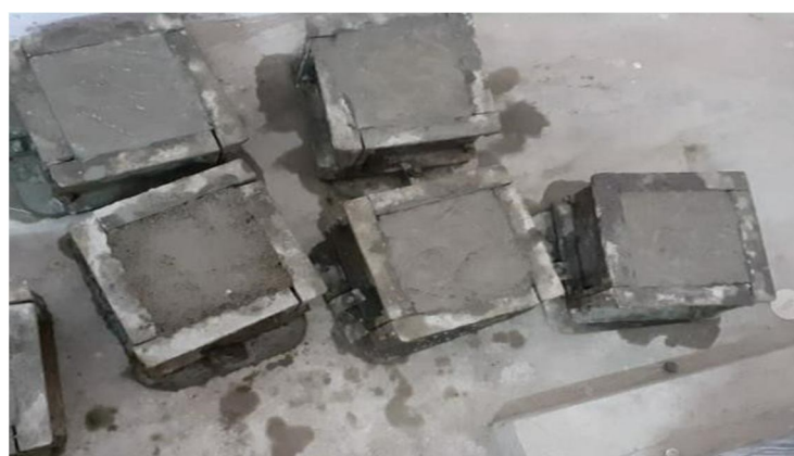
Fig 20: Cubes after Filled with concrete
