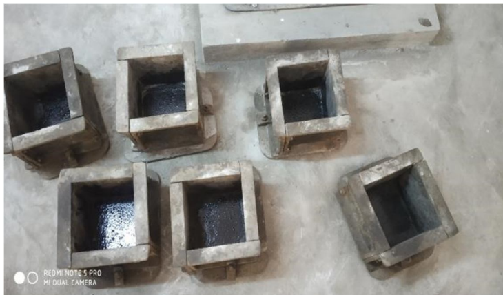
Fig 19: Cubes after applying grease
