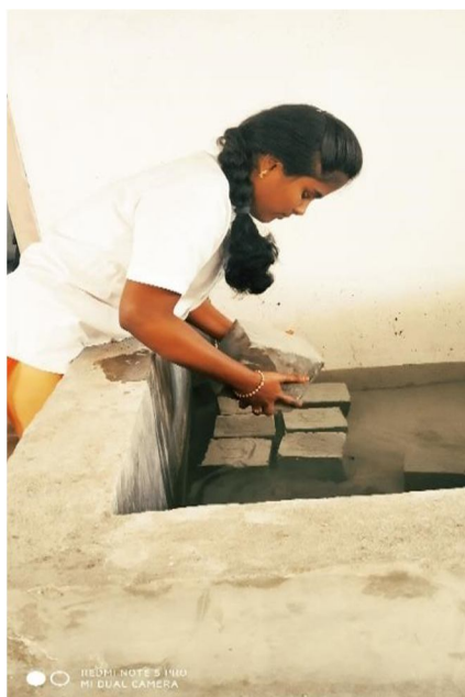
Fig 26: placing cubes for curing in curing Tank
