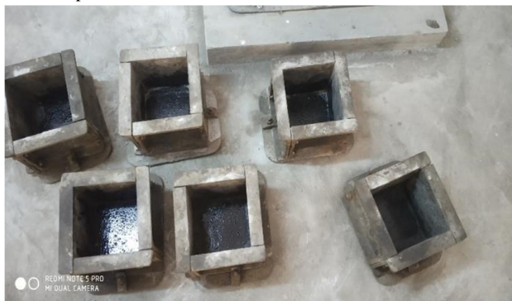
Fig 19: Cubes after applying grease
