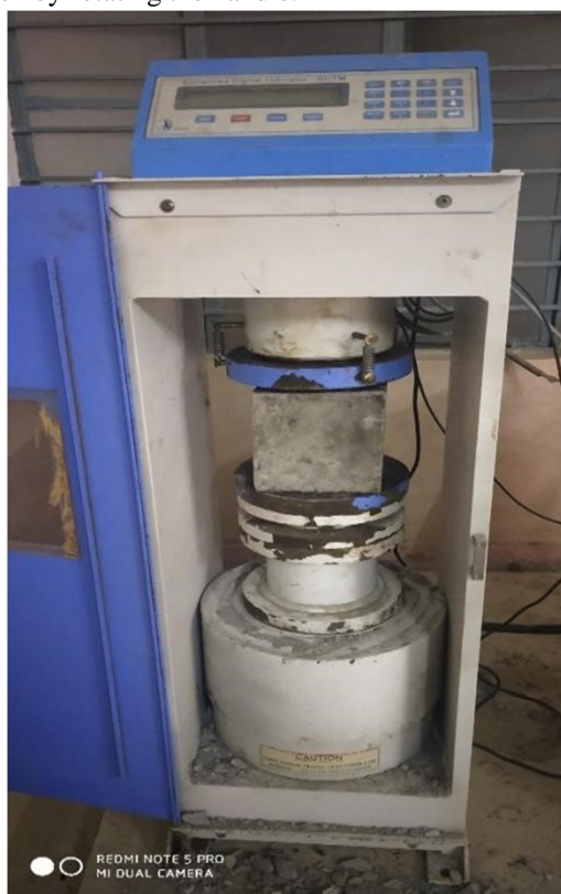
Fig 27: placing specimen for compression value
