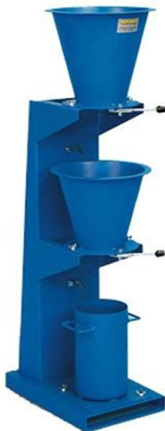
Fig 17: compaction factor test
