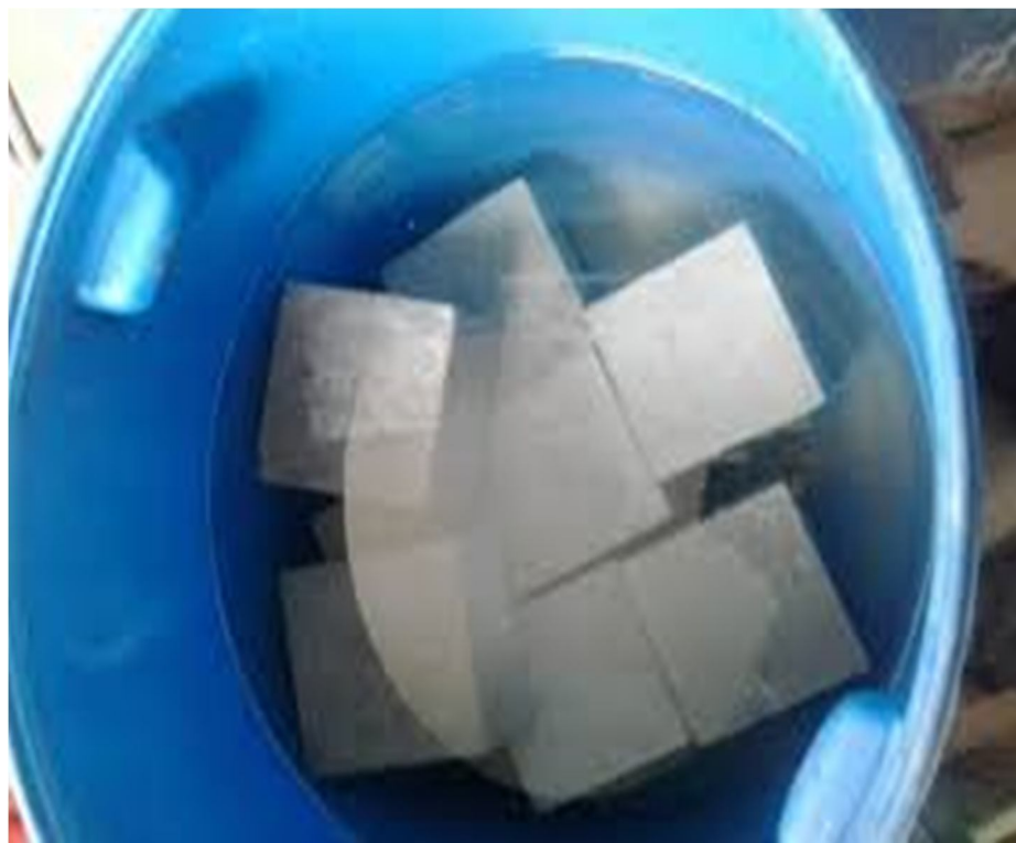
Figure 5 Curing of Samples
