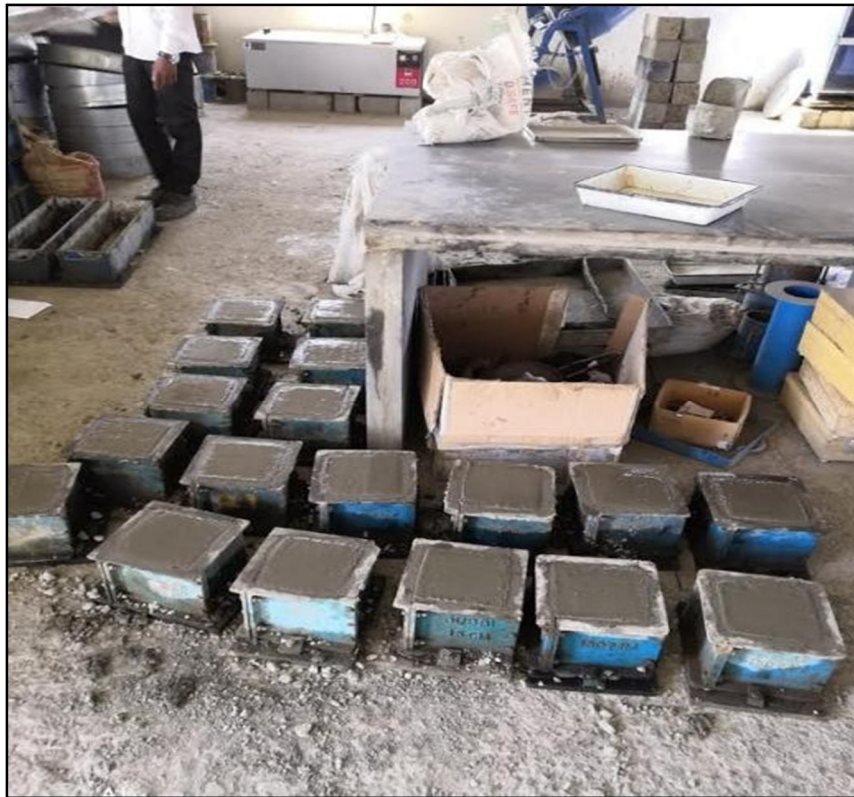
Figure 4 Casting of Cubes and Beams
