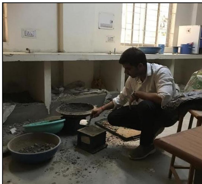
Figure 3 Sample Prepared with M-sand and Bamboo fiber
