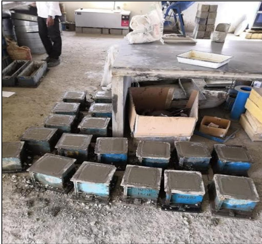
Figure 4 Casting of Cubes and Beams
