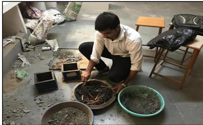
Figure 3 Sample Prepared with M-sand and Bamboo fiber
