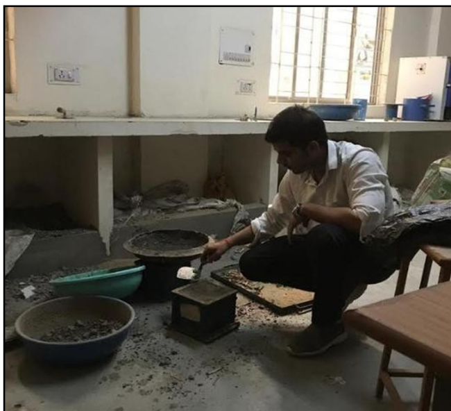
Figure 3 Sample Prepared with M-sand and Bamboo fiber
