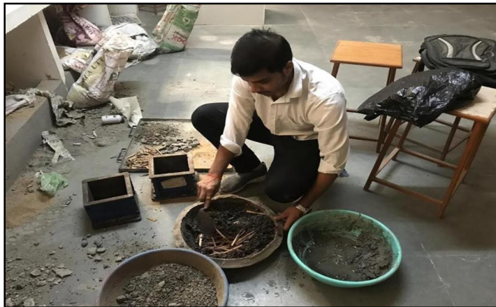
Figure 3 Sample Prepared with M-sand and Bamboo fiber
