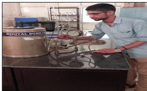
Fig: 1.5 Setup of bomb calorimeter
