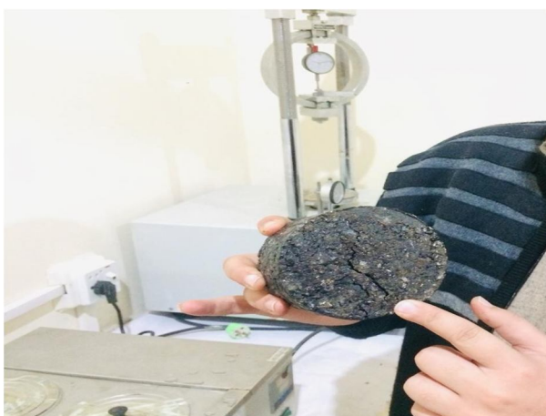
Crack after IDT testing
