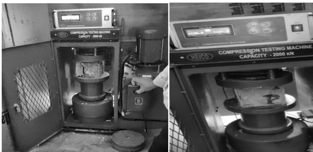
Figure 5: Shows the compressive strength test on Cubes
