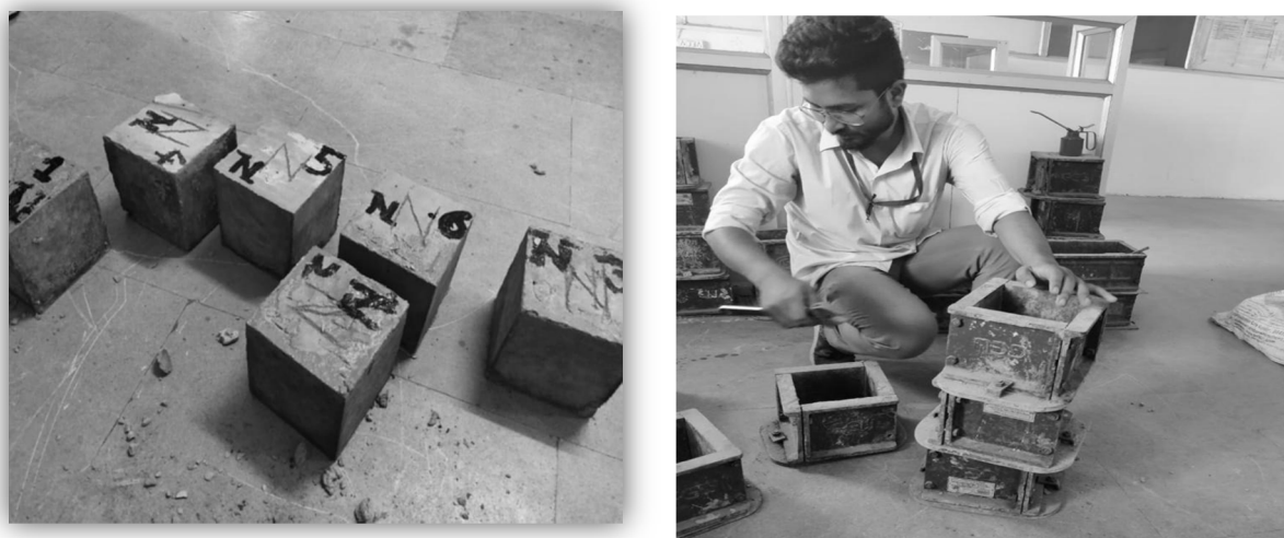
Figure 4: Shows the Concrete Cubes
