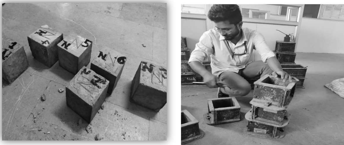
Figure 4: Shows the Concrete Cubes
