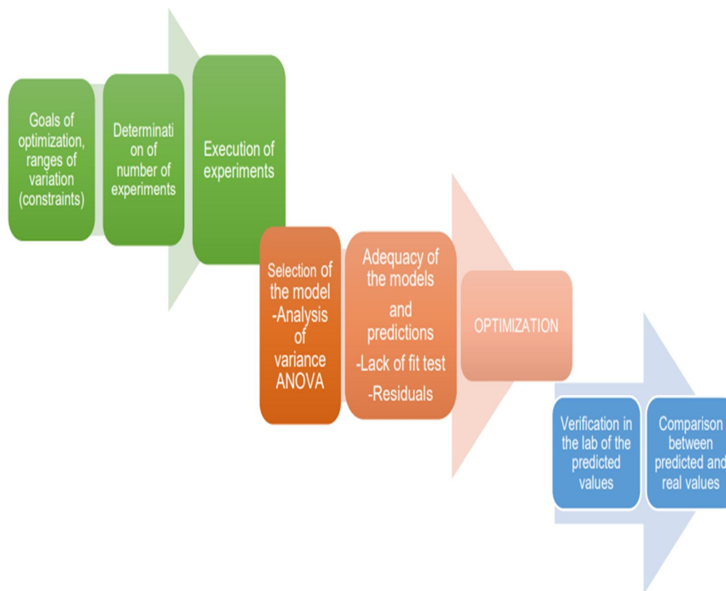
Figure 3: Mixture design process, adapted from Anderson and Whitcomb (2005) and Kharazi (2013).
