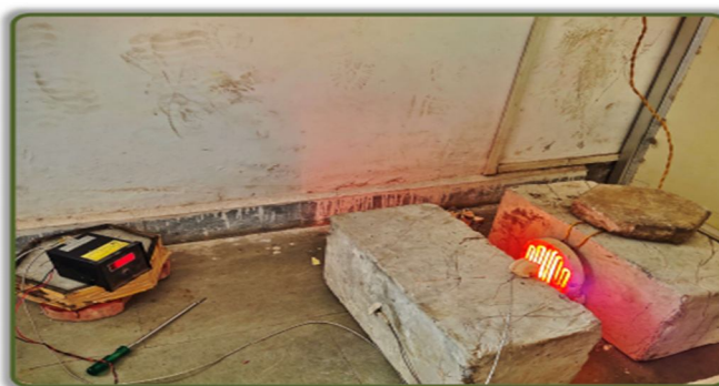
Figure 9 Thermal conductivity measurement
