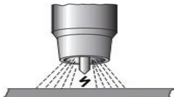
Figure (2.7): High frequency ignition
