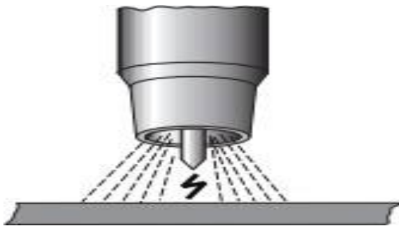
Figure (2.7): High frequency ignition
