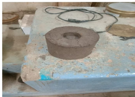
Fig 3 : California Bearing Ratio Test
