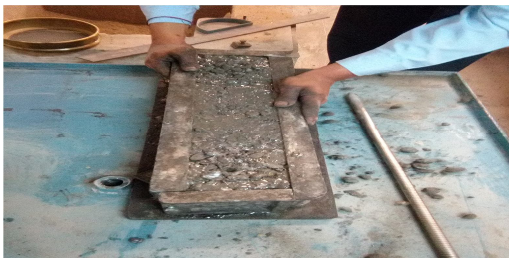
Fig. 4.16 Casting of slab
