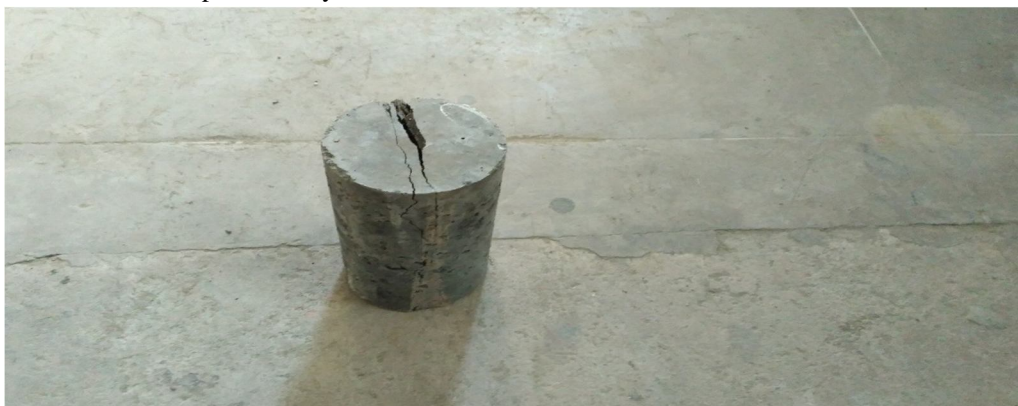
Fig. 4.13 Failure of cylinder with fiber
