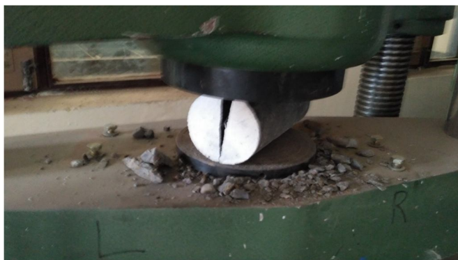
Fig. 4.9 Brittle failure of cylinder without fibre
