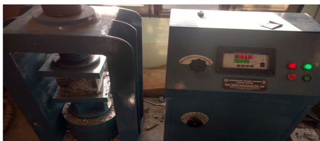
Fig. 3.1 Compression Testing Machine
