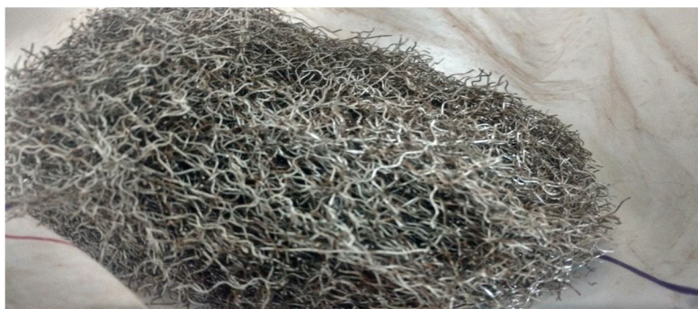
Fig. 3.2 Steel fiber used in project
