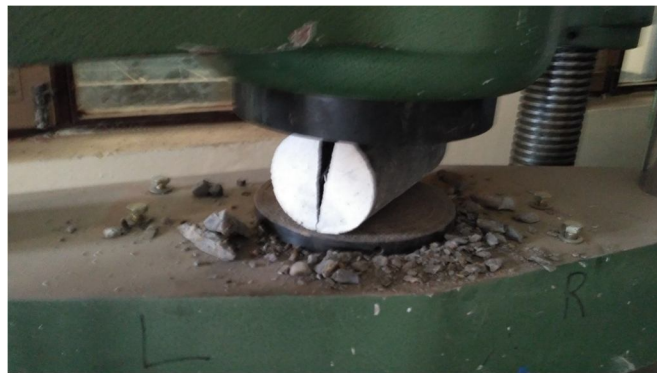
Fig. 4.9 Brittle failure of cylinder without fibre
