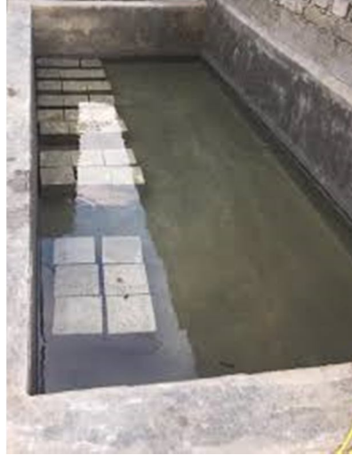
Fig. 3.4 Curing of cubes
