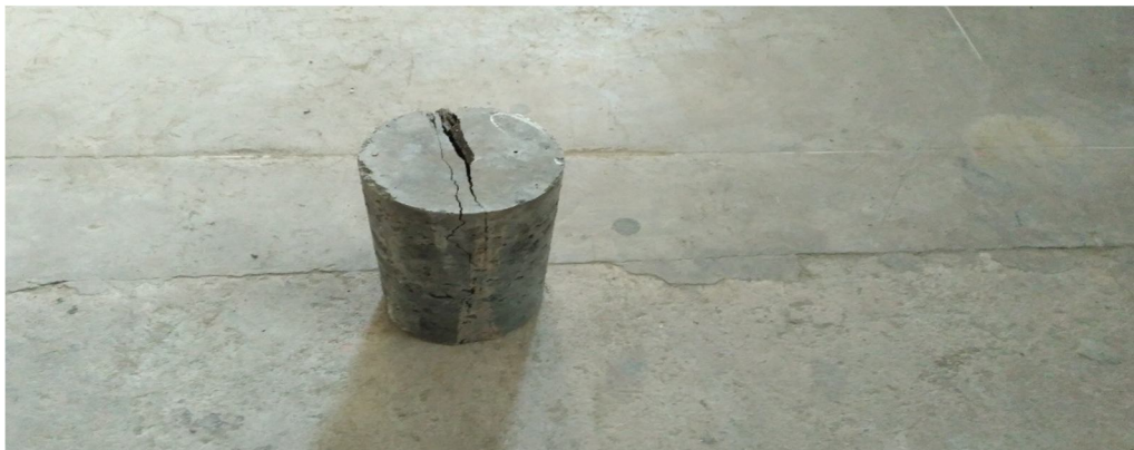
Fig. 4.13 Failure of cylinder with fiber
