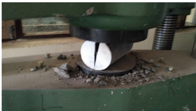
Fig. 4.9 Brittle failure of cylinder without fibre
