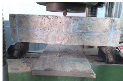
Figure 4 Experimental setup of combination of both PCC & SCC beam and its crack formation (PCC layer above).
