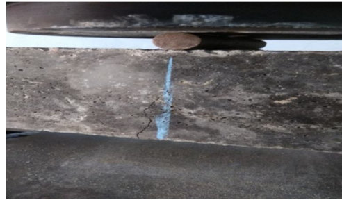
Figure 2 Experimental setup of SCC beam and its crack formation.
