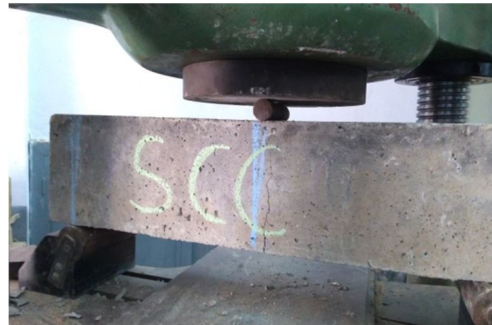
Figure 2 Experimental setup of SCC beam and its crack formation.
