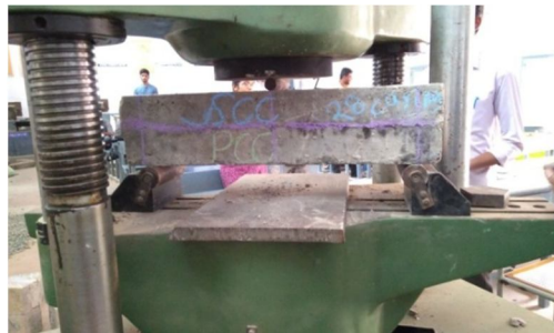
Figure 3 Experimental setup of combination of both PCC & SCC beam and its crack formation ( SCC layer above).
