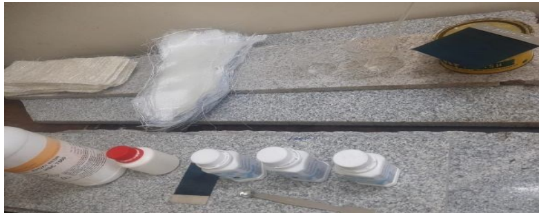
Fig 1 : Glass Fibre, Epoxy resin, Hardner and MWCNTs, Nanoclay and ZnO
