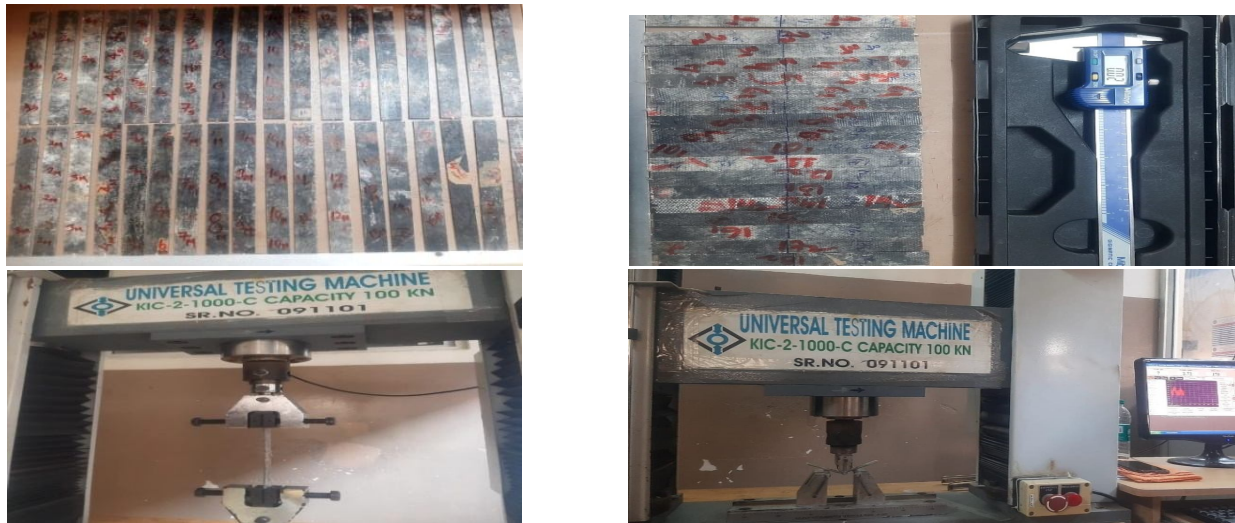
Fig 6. : Tensile test for Specimens in UTM as per ASTM Standards. Fig 7 : Flexural bending test for Specimens in UTM as per ASTM Standards.
