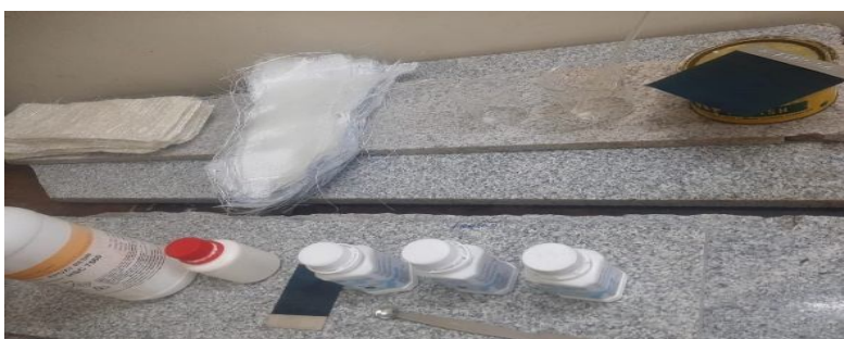
Fig 1 : Glass Fibre, Epoxy resin, Hardner and MWCNTs, Nanoclay and ZnO
