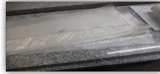
Fig 2 : 09 layers Stacking sequence arrangement of Bi-directional and chopped stranded glass fibre mat
