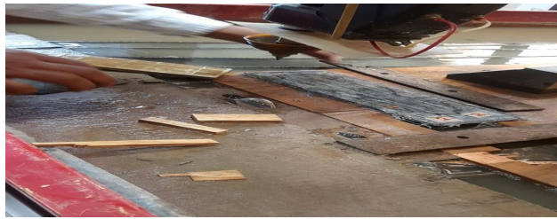
Fig 5 : Abrasive Waterjet Cutting of Specimens to standard dimensions for Tensile & Flexural Test
