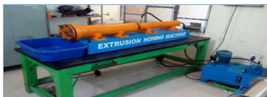
Fig 1: One - Way type extrusion honing Machine.
