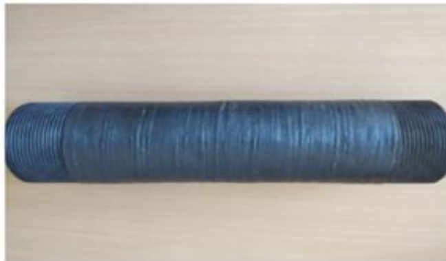
Fig -8: Twisted shaft
