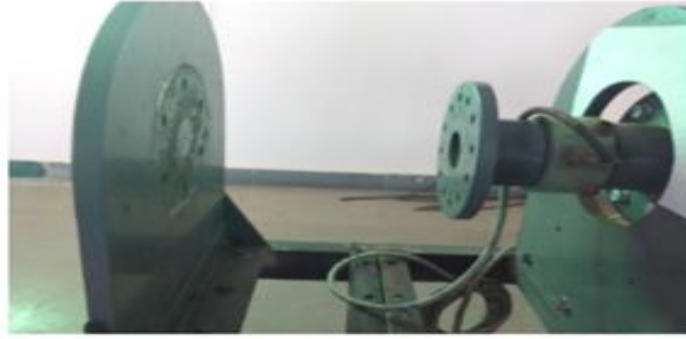
Fig -7: Torsion testing setup
