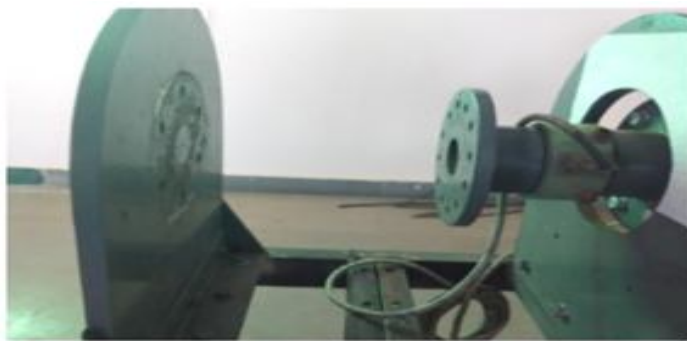
Fig -7: Torsion testing setup
