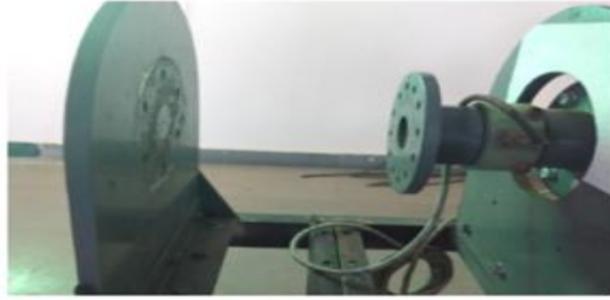
Fig -7: Torsion testing setup
