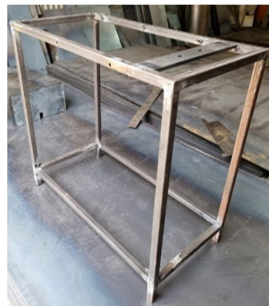
Fig.10 Model & Actual Photo of Foundation Frame
