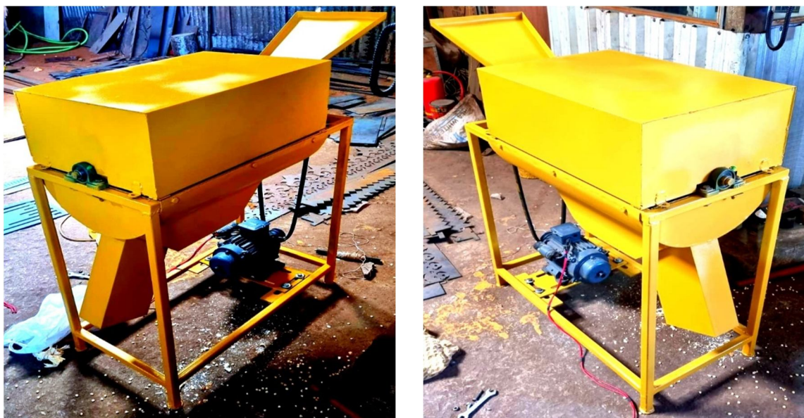
Fig 2 Final Assembly of Corn Sheller
