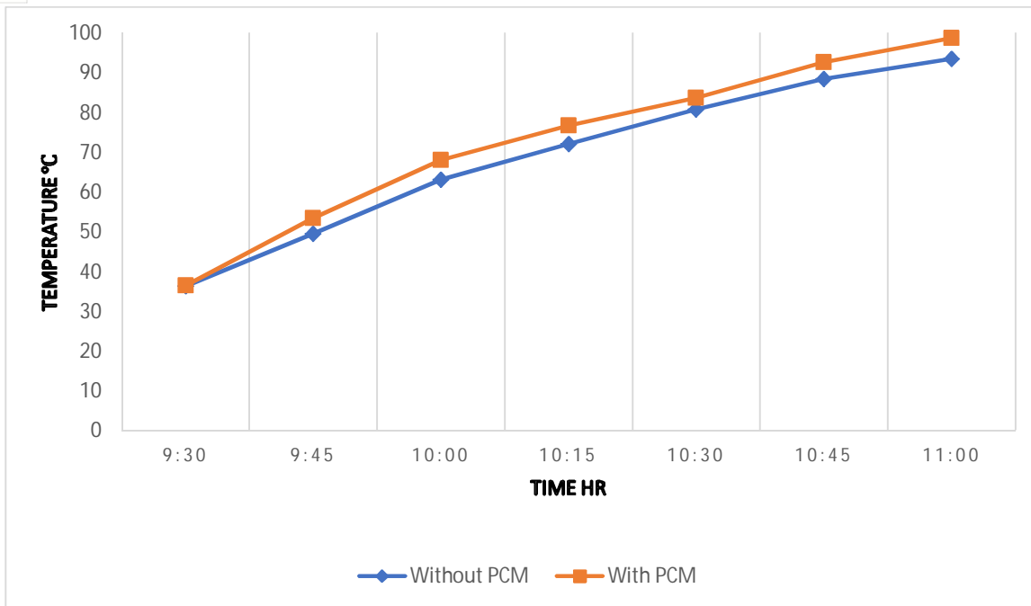
Fig.- 4 Variation of water temperature inside the pot during heating test with time
