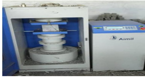
Fig.3.7 Testing of Compressive strength
