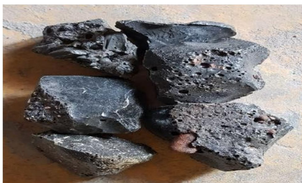
Fig -1: 20mm Lump sized of Cupola Slag aggregate
