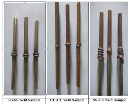
Fig 2 Friction welded dissimilar welded specimens
