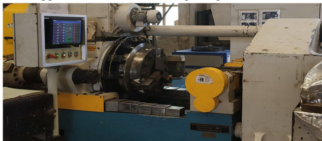
Fig 1 Continuous Drive Friction Welding Machine
