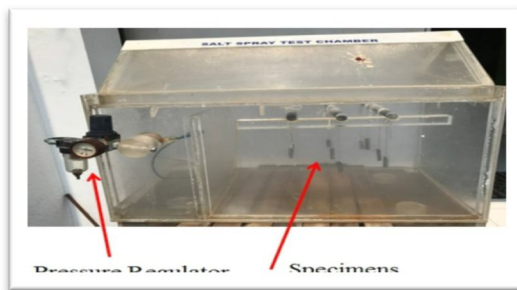
Fig 12 Salt spray corrosion setup
