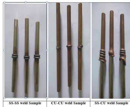
Fig 2 Friction welded dissimilar welded specimens
