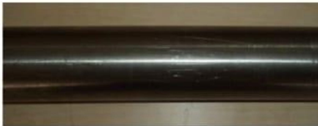
FIGURE: EN19 alloy steel
