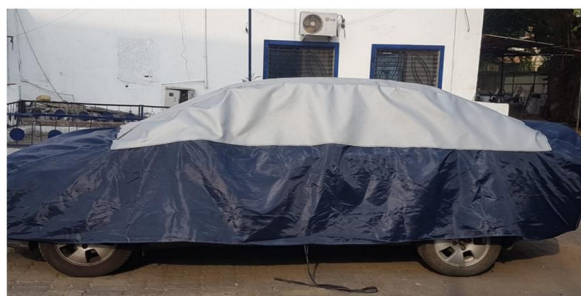
Fig 6 Sedan vehicle covered with heat-resistant roof-top double-sided silicone-coated fibreglass cloth
