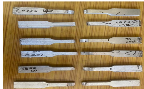
Fig 2– Work specimens after tensile test on UTM
