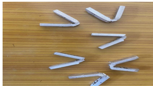
Fig 5 – Work Specimens after Impact Charpy test
