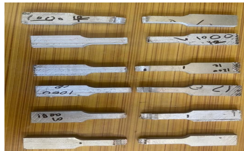
Fig 2– Work specimens after tensile test on UTM
