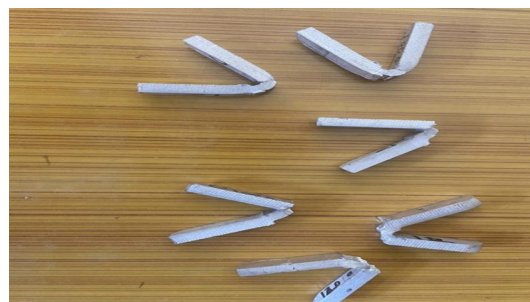
Fig 5 – Work Specimens after Impact Charpy test
