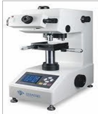
Figure 7: Vickers Hardness Test Equipment
