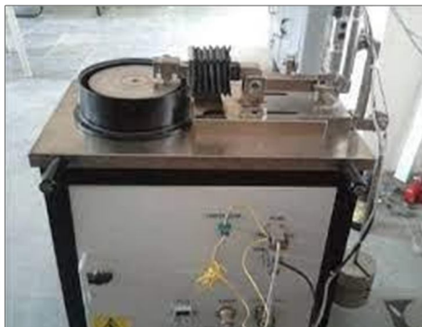
Figure 5: Wear Test Equipment
