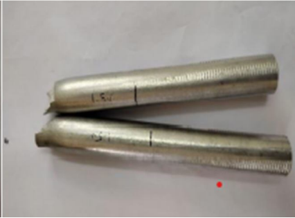
Figure 8: Tensile tested Al6061 + 1.5% ZrO 2 specimen
