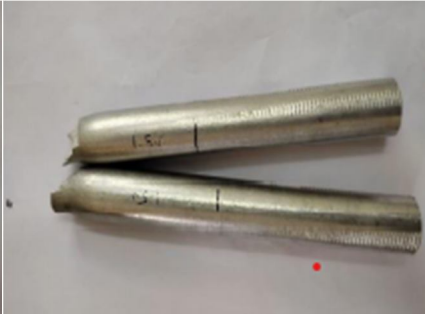
Figure 8: Tensile tested Al6061 + 1.5% ZrO2 specimen
