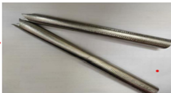
Figure 6: Tensile tested Al6061 + 0.5% ZrO2 specimen
