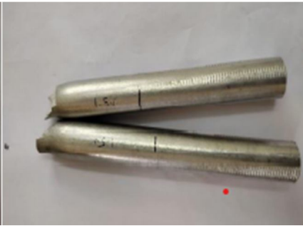
Figure 8: Tensile tested Al6061 + 1.5% ZrO 2 specimen
