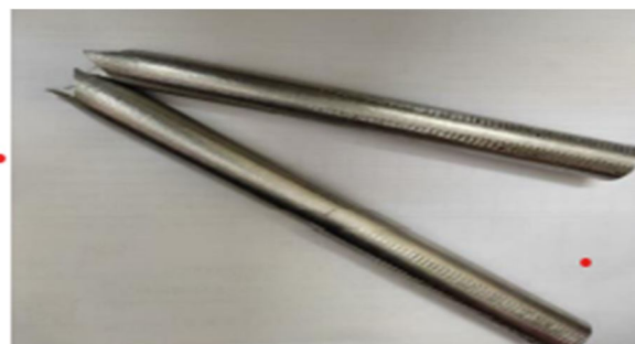
Figure 6: Tensile tested Al6061 + 0.5% ZrO2 specimen
