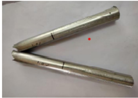
Figure 7: Tensile tested Al6061 + 1.0% ZrO 2 specimen
