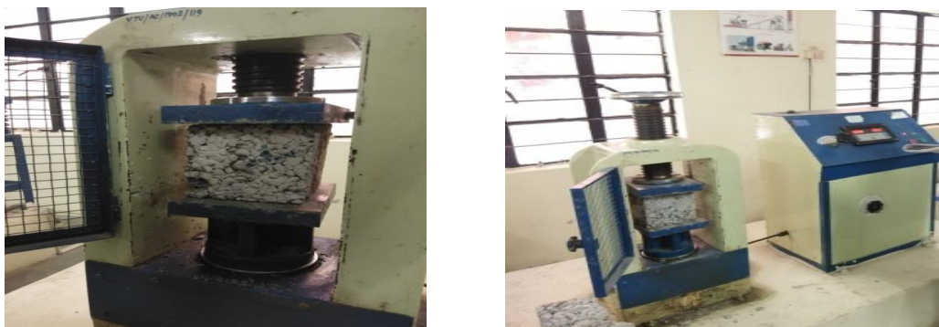
Fig 1.1 Compressive strength test of cube
