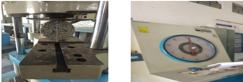
Fig 1.2 Split Tensile Strength of Concrete
