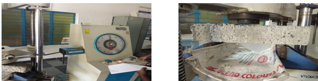
Fig 1.3 Flexural Strength of Concrete
