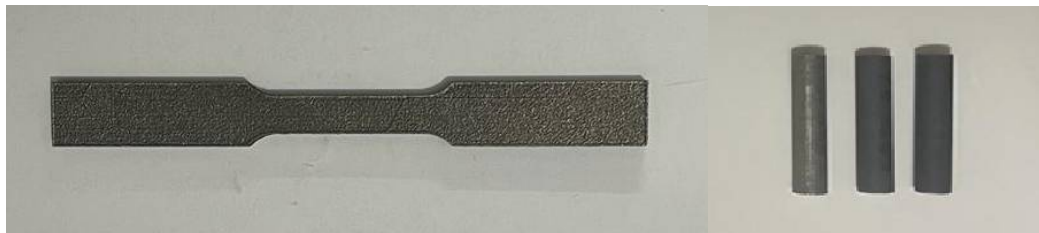
Fig 3 (a) Tensile test specimen and (b) Wear test specimens
