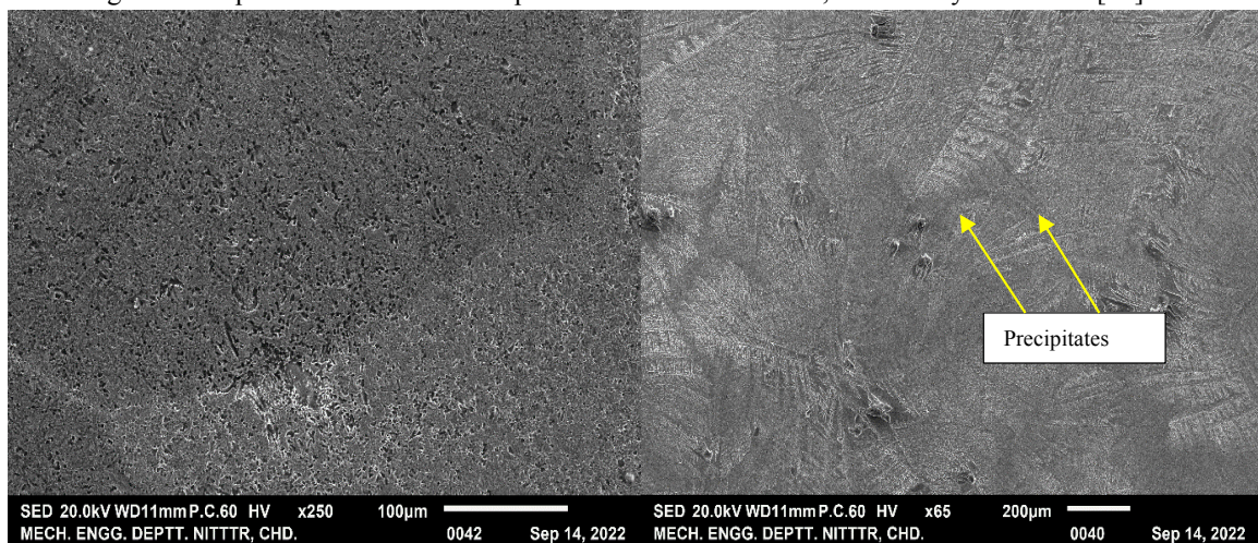
Fig 4 (a) SEM micrographs of HT 1 specimens (b) Precipitates formation
