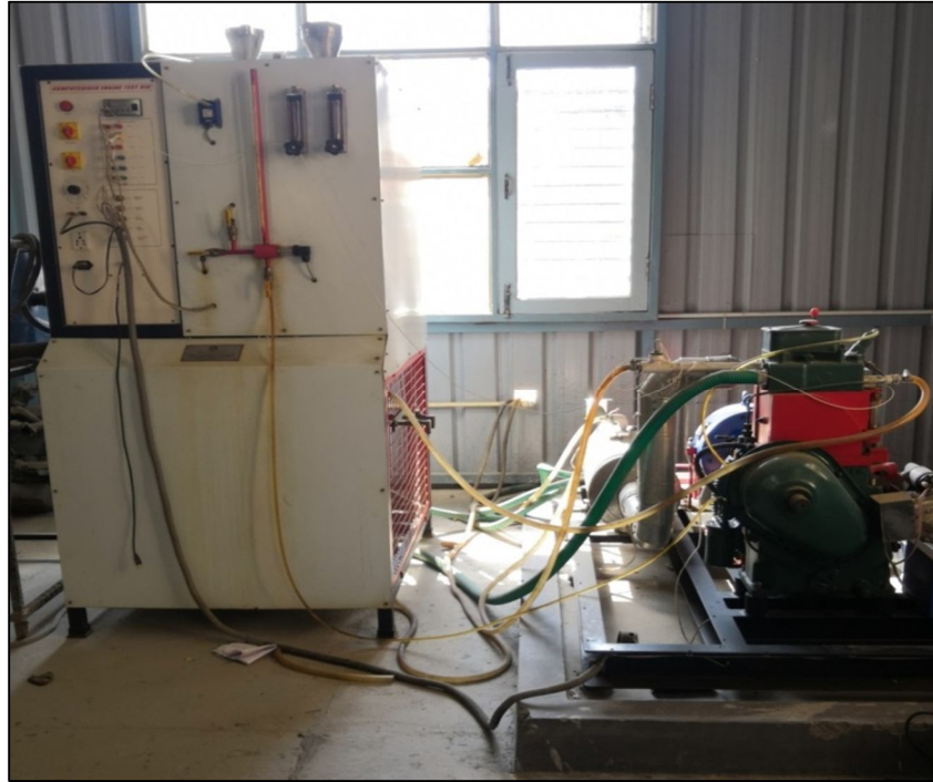
Figure 1a Kirloskar Diesel Engine Set-Up
