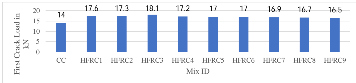
Figure 4.6 Bar Graph of First Crack Load of CC and HFRC Beams
