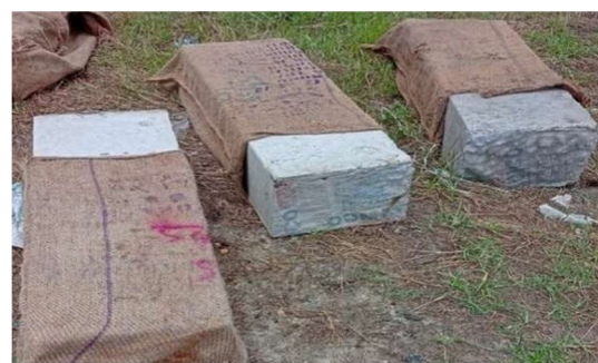
Fig 15 Curing of Beam
