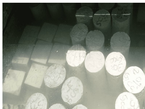
Fig 12 Curing of Specimen
