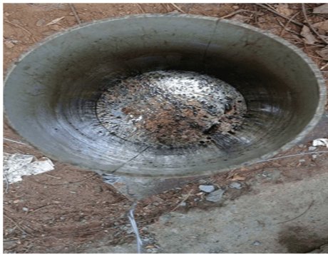
Fig 10 Greasing of Mould
