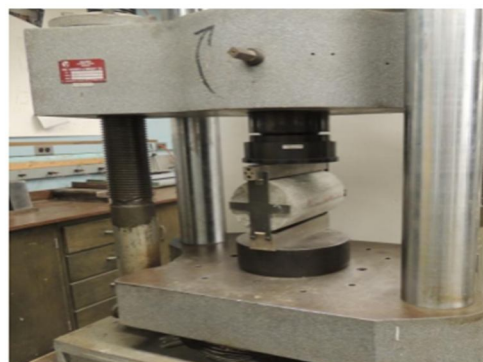
Split tensile strength setup
