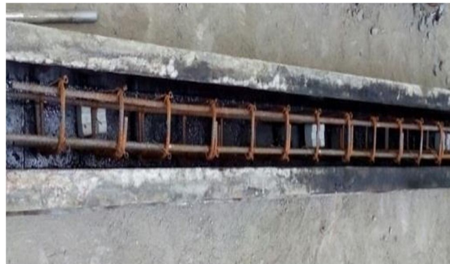
Beam Specimen with Reinforcement
