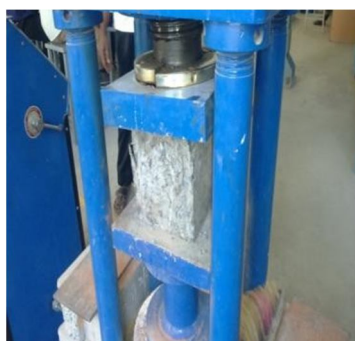
Compression Test on Cube
