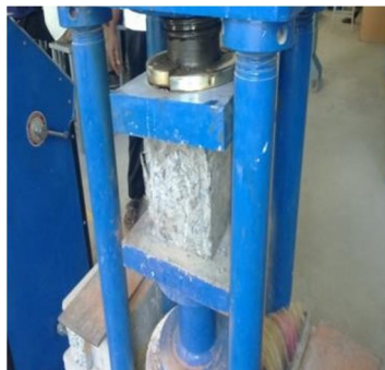
Compression Test on Cube
