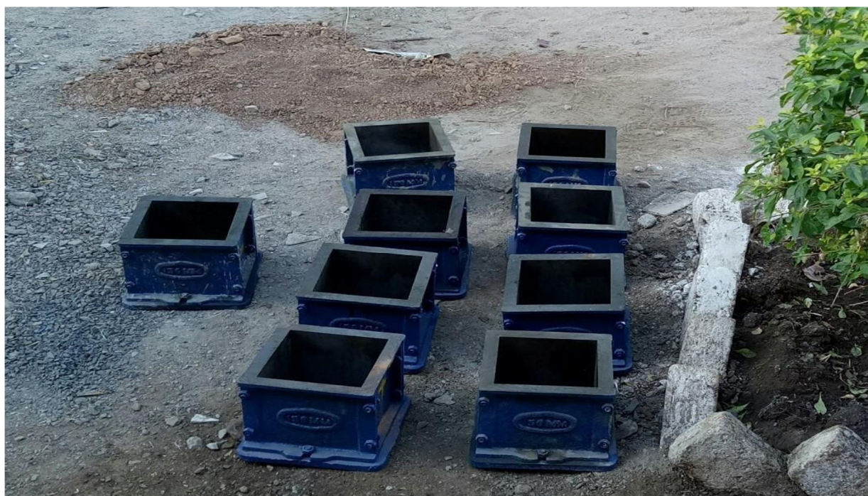
Fig.1 - Mould for casting
