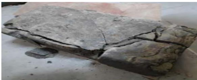
Fig: Brick after the compressive strength test, failure due to compressive load
