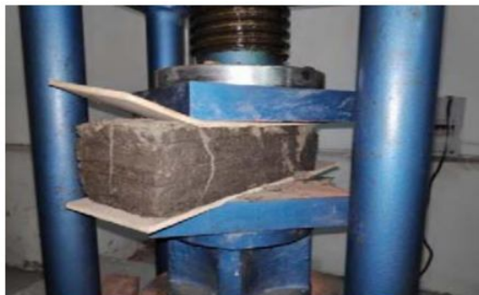
Fig: Compression strength test on brick to determine the load carrying capacity of bricks under compression
