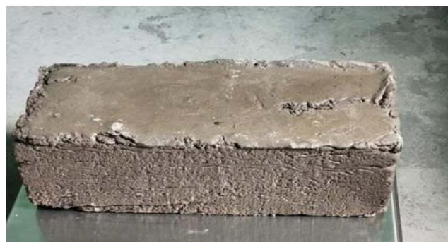
Fig: Plastic Sand Brick after removing it from the mould
