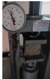
Figure 6- Compressive Strength Test of Concrete Cube
