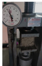
Figure 6- Compressive Strength Test of Concrete Cube
