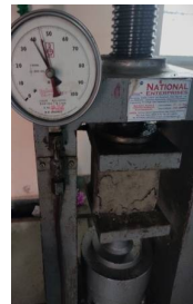
Figure 6- Compressive Strength Test of Concrete Cube
