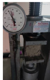
Figure 6- Compressive Strength Test of Concrete Cube
