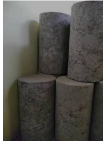
Figure 7- Concrete Cylindrical specimens
